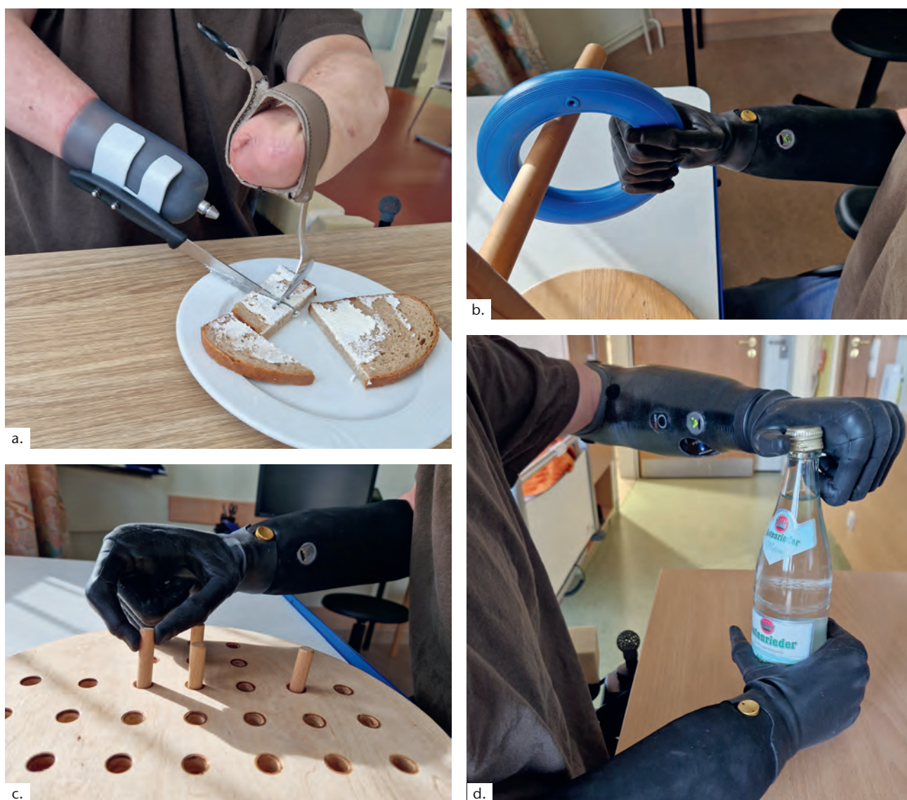
Fig. 5a–d The knife is securely attached and, in combination with a cuff for the fork, independent eating is made possible (a). Targeted grasping and releasing provides experience in controlling the prosthesis and its components (b). By using objects of different sizes and shapes, prosthesis wearers train various grips and the controlled use of force (c). Bilateral ADL training enables the use of prostheses in everyday situations (d).
