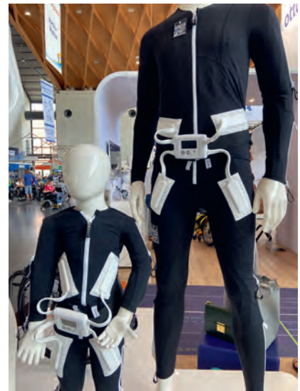
Fig. 7 Neuromodulation whole-body compression and e-stimulation orthoses utilize the principle of sensory stimulation through compression and electrical stimulation with multiple effects on the addressed muscles.
