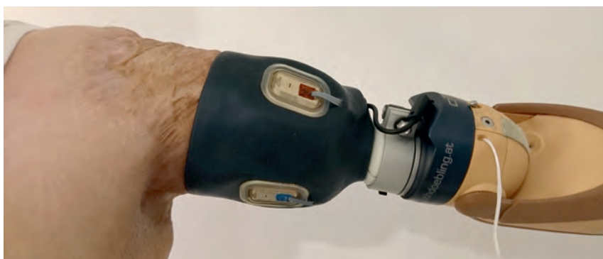
Fig. 3 Possible design for an "electrode socket" that encloses all necessary surface electrodes for prosthesis control following successful TMR surgery (supplied by OTH Döbling, Vienna, Austria).
