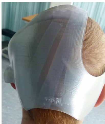
Fig. 2 Trial fitting of an individual head protection helmet, produced with PETG using the FDM process.
