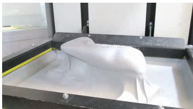
Fig. 3 Deep drawing the heated material over the processed model.
