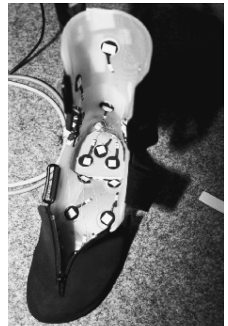
Abb. 2 Special orthosis made for testing.
