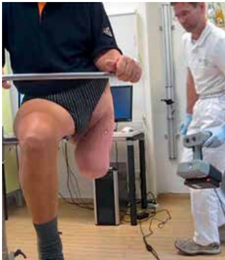
Fig. 3 Shape determination with video-based scan.
