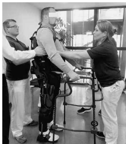
Fig. 4 Rollator for the first therapy session in the Ekso. The image shows a patient with spinal cord injury below C7, ASIA A. The legs and torso are well secured and the body's centre of gravity remains in the middle even if the patients are very large and heavy.
