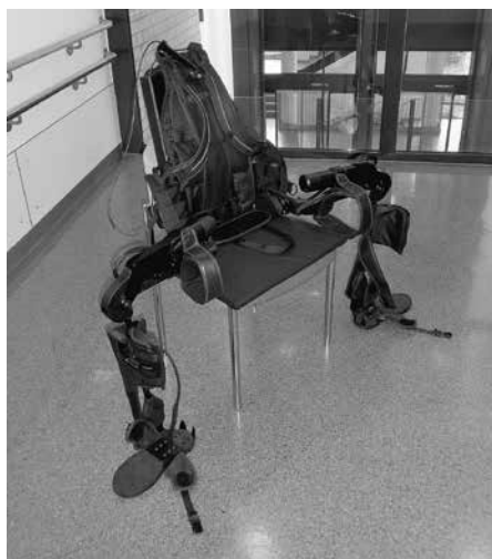
Fig. 3 The Ekso in the initial position for transferring the patient from the wheelchair to the device; the "legs" can be adducted after transfer. The well padded clamps for securing the patient and the firm back plate are also visible.
