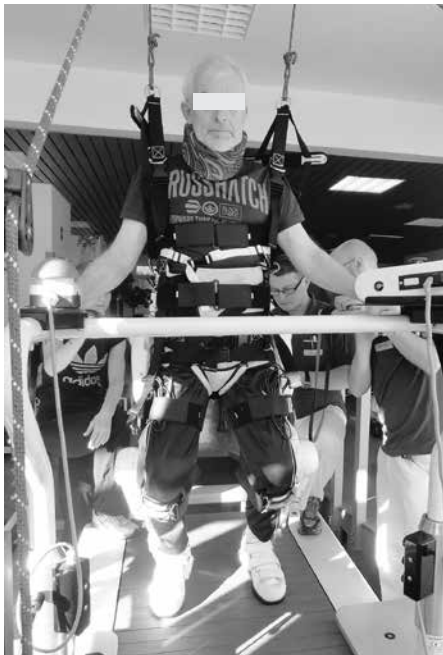
Fig. 6 Resting phase in the HAL: Using the Woodway, the patient can hang in the straps to rest. The patient must actively extend the hip and knee joints to stand up.
