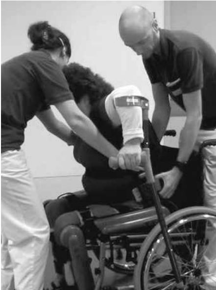
Fig. 1 Standing up with the ReWalk: The arms must be positioned far to the rear and the torso must be bent forward. The ring-like devices for securing the forearm crutches cause painful pressure at the bends of the elbows.
